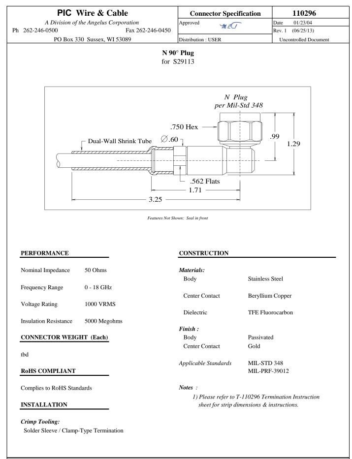
PIC Wire & Cable Connector User specification sheets are non-controlled documents. Please contact PIC Wire and Cable or visit the PIC website (www.picwire.com) to ensure the latest revision of the drawing is being viewed.
