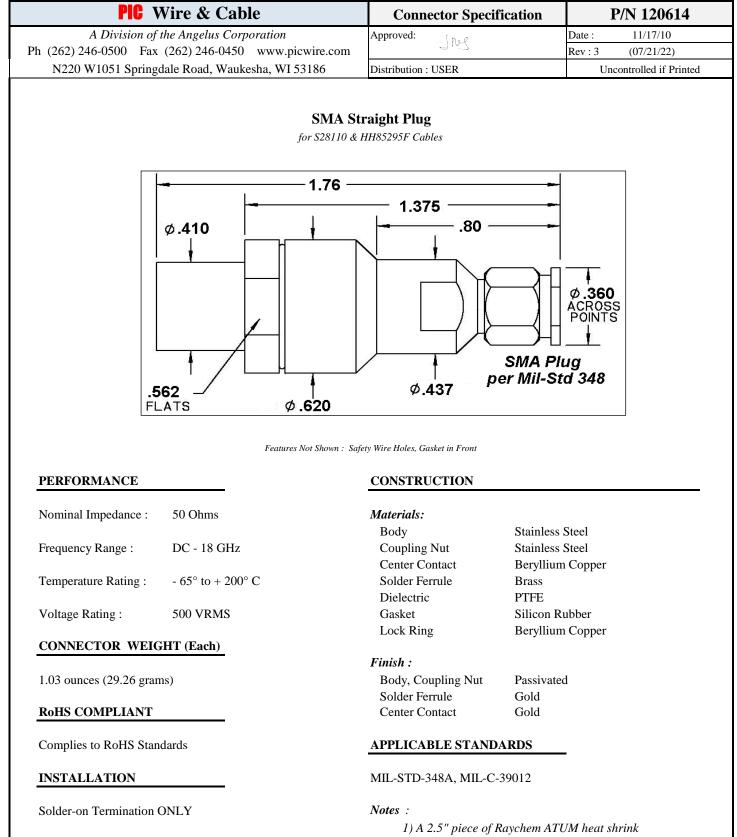
*P/N ATUM-16/4-0 provided with connector for purpose of strain relief & moisture protection.*
