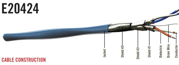
Conductors: Silver-Plated Copper Dielectric: Dual Layer FEP Shield #1: Aluminum/Polyester Foil (each pair) Drain Wire: Tin-Plated Copper Shield #2:Aluminum/PolyesterShield #3:Silver-Plated Copper BraidJacket:FEP, Translucent Blue
